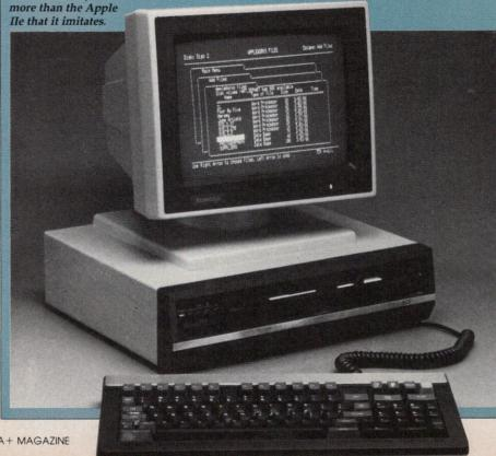
a detached keyboard, a system unit that houses the disk drives and CPU, and a monitor. Internally, the Ace features a 65C02 processor, 128K of RAM, a 67-watt power supply (the Apple IIe's is 35 watts), two Applecompatible expansion slots, and a built-in fan. It has internal connectors for Franklin-supplied RAM expansion, RGB video (which requires a \$79 interface card), and a 16-pin joystick. The Franklin's video ROM generates either standard Apple- or Mousetext-compatible character sets.
